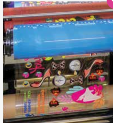
Laminazione automatica transfer UV DTF (film A+B) Automatic UV DTF transfer lamination (A+B film)
